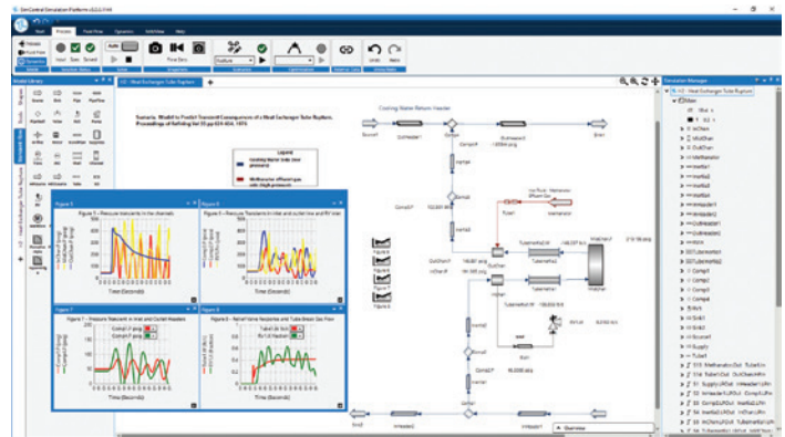
Figure 2: AVEVA Process Simulation user interface with Process, Fluid Flow and Dynamic modes, the Process library opened up and showing a dynamic trend while in process mode. A snapshot manager helps manage scenarios.
