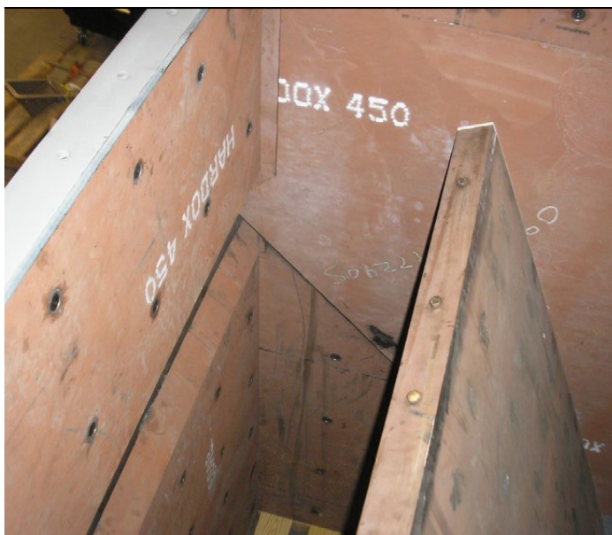
Figure 6. This liner is made with an abrasion-resistant steel.
