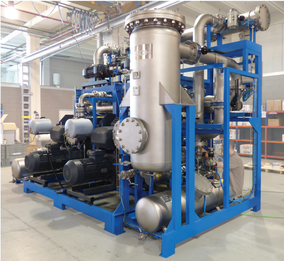
Figure 3: Vacuum system with two Huckepack once-through oil-lubricated rotary vane vacuum pumps for chemical applications
