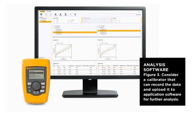
It also records the pressure applied to the valve control element from 4 to 20 to 4 milliamps looking for smooth linear changes in pressure across the band ascending and descending.
