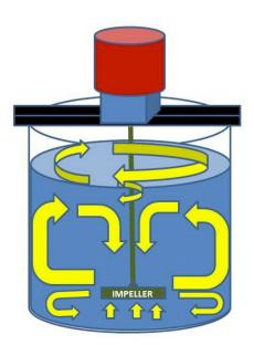
**SUFFICIENT FLOW** Figure 6. Impeller is well covered and close enough to the vessel bottom to reach lower areas of vessel to prevent settling.
