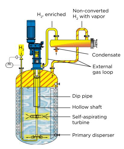
**COMBINED GASSING WITH EXTERNAL GAS LOOP** Figure 3. This shows an example of hydrogenation with water (vaporous) as a byproduct.
