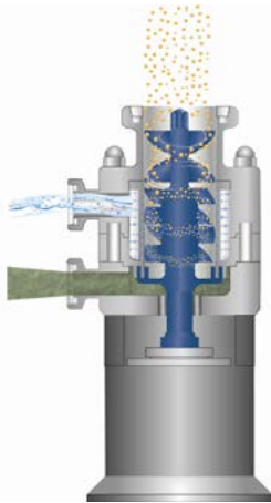
Figure 2. The module mixes, homogenizes and disperses solid and liquid phases in a single pass.
