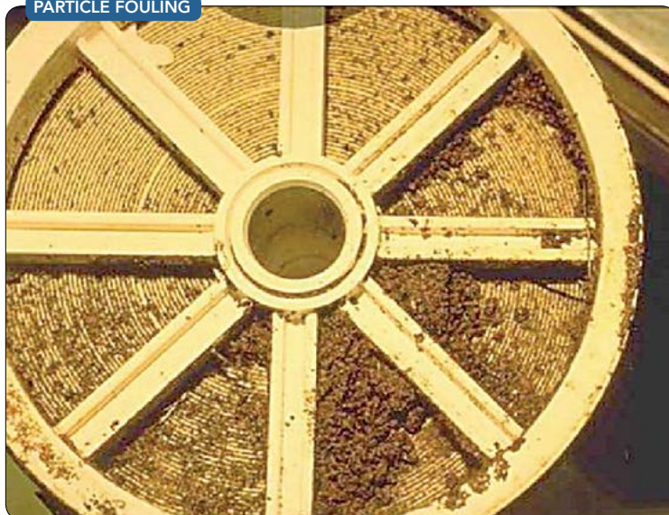
Figure 2. Such fouling occurs in the first RO stage, particularly on its feed screen.
