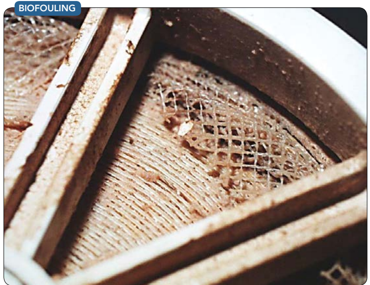
Figure 4. Both the first and second stages of a system can suffer from such fouling.
