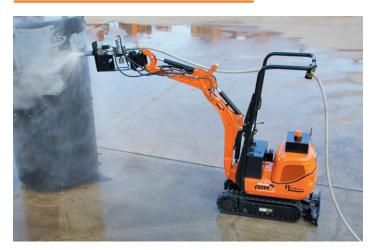
Since semi-automated systems are directed by remote control, or from a cab, they allow operators to keep their distance from the high-pressure water and any flying debris. This exposes the operator to less risk (and fatigue) than holding a high-pressure lance and makes it easier to comply with OSHA personal protective equipment (PPE) requirements.
