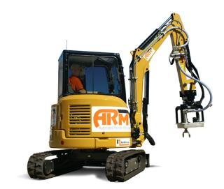
systems with multi-application capabilities. These typically have articulated arms mounted on commercial excavators, with changeable tooling designed to accomplish specific tasks.
