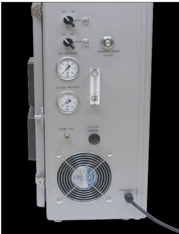
System for generating Ozone into the convey line
