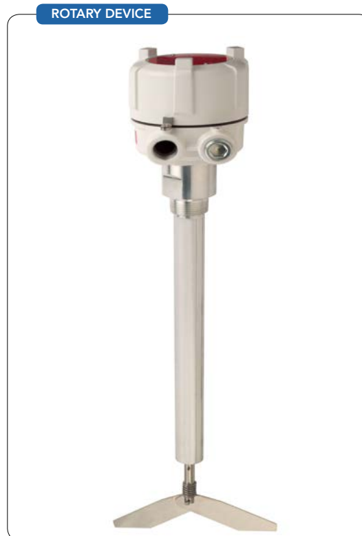
Figure 1. For high-level detection in a tank, a rotary is mounted on top of the tank, and a custom-fabricated extension places the paddle at the desired level.
