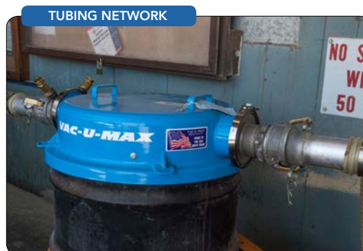
Figure 4. This vacuum system uses individual tubing networks to quickly and easily move from one tubing network to the next, providing the convenience of a multi-inlet central vac, with the energy efficiency and flexibility of a portable vacuum. Source: Air Cleaning Technology
