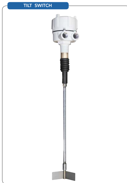
Figure 4. A top-mounted tilt switch is used for high-level detection, activating an alert when the material tilts the switch by 15°.
