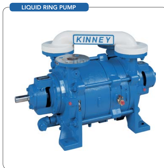
Figure 1. A liquid ring pump relies on handling the process fluids as a vapor at inlet and condensing them to the liquid phase while passing through the pump.
