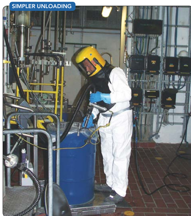
Figure 2. Vacuum conveyor wand eases unloading of a hazardous chemical. Source: Volkmann.
