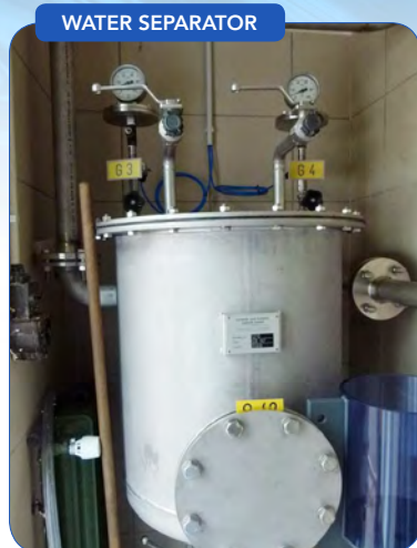
Figure 4. Here, the gas inlet with first water separator is shown.
