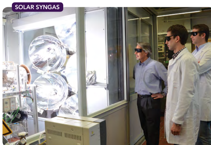
Figure 3. Process uses concentrated sunlight to convert carbon dioxide and water into a syngas that then is used to make kerosene. Source: ETH Zurich.
