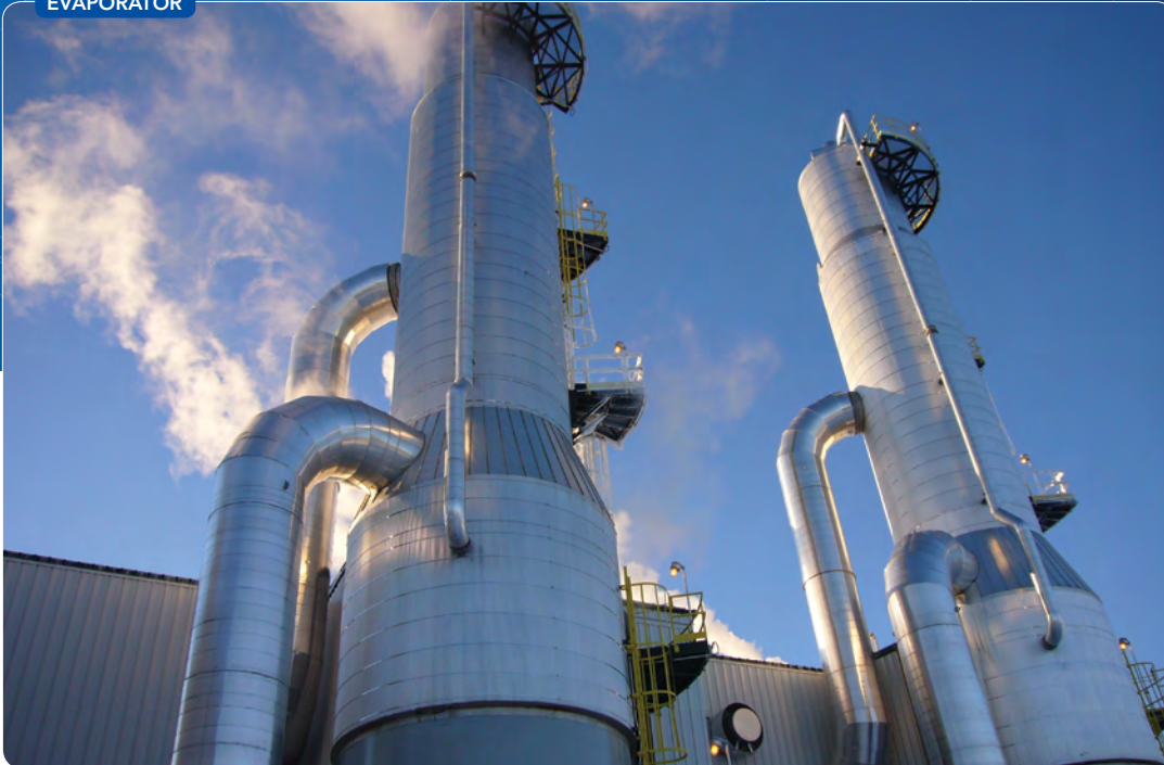
Figure 1. Plants are opting for evaporators to handle certain wastewaters even though they aren't the lowest cost option. Source: GE Power & Water.
