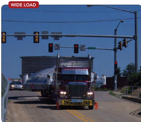
Figure 1. This wide load represents only one section of a large vessel that will require field assembly.
