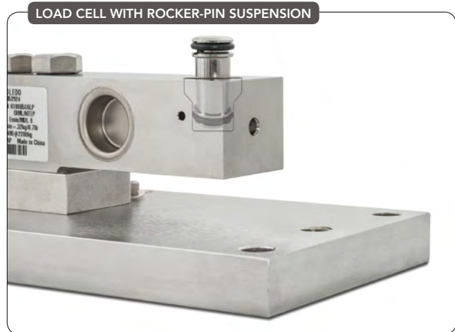
Figure 1. A self-aligning rocker-pin suspension design allows some degree of movement to occur without causing damage to the load cell or changes to its accuracy.
