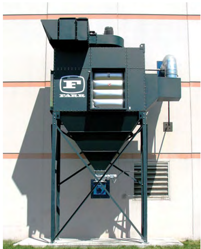
This heavy duty dust collector with explosion vent is designed to survive a combustible dust explosion with minimal damage.
