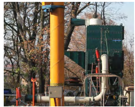
At the startup of a staged explosion, explosive dust is injected into the dust collector to create a flammable cloud.
