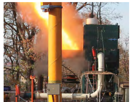
The flame is diverted away from the dust collector to a safe area.
