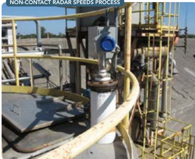
Figure 1. This continuous non-contact radar level meter eliminates the need for operators to conduct multiple manual inch counts each day, reducing cycle times and worker exposure to chemical vapors.
