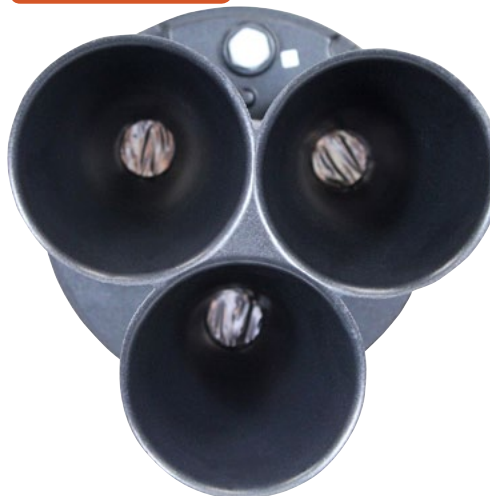
Figure 3. Using three transducers to continuously measure and map the material surface helps ensure accuracy.
