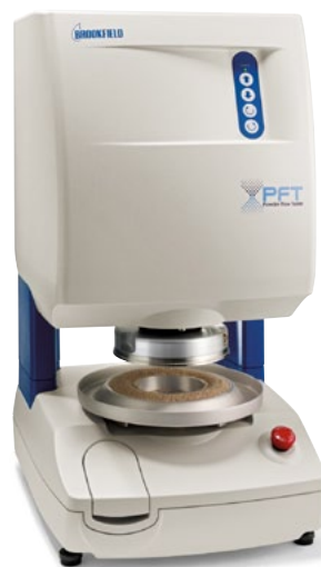
Figure 2: The shear cell containing the powder sample is placed in a powder flow tester.
