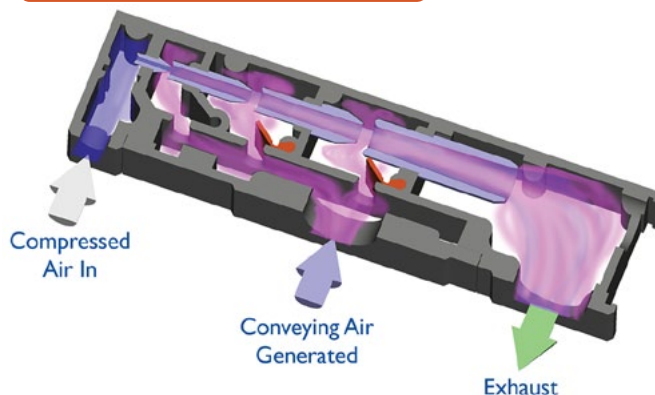
Figure 4: Multiple stage ejector pumps like the Multijector for Volkmann are frequently used in vacuum conveying.
