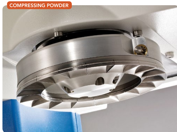
Figure 3: A vaned lid compresses the powder sample in the shear cell, causing powder particles to fill the compartments in the vaned lid.
