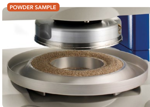
Figure 1. Shear cell technology can easily test powders for time consolidation.
