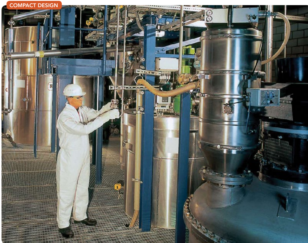
Figure 3: This vacuum conveyor (front, right) allows the bulk material receiver to be mounted directly above and feeds powders into the process vessel beneath.
