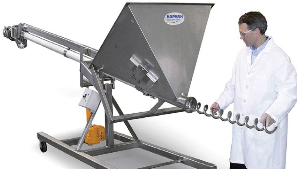
Figure 3. Author shows how tilt-down design makes screw removal easy.
