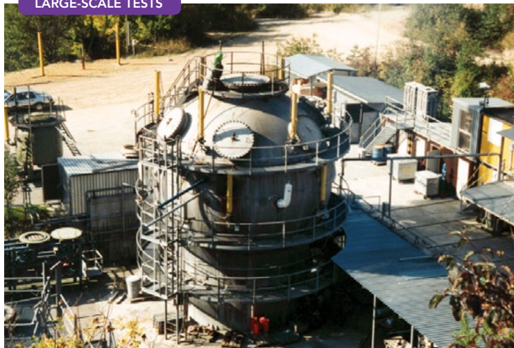
Figure 9. A 250-m 3 explosion test chamber fitted with Fike 50 L suppressors (white colored containers) is used for large-scale testing.
