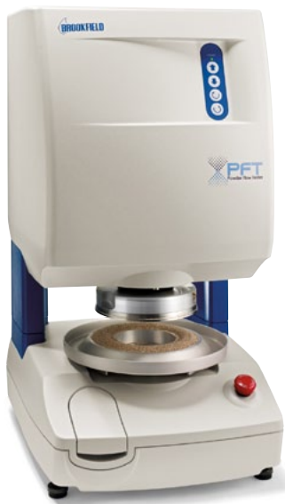
Figure 1: This powder flow tester from Brookfield can access a powder's flow behavior and can discern differences in powder "failure strength" as a function of relative humidity.
