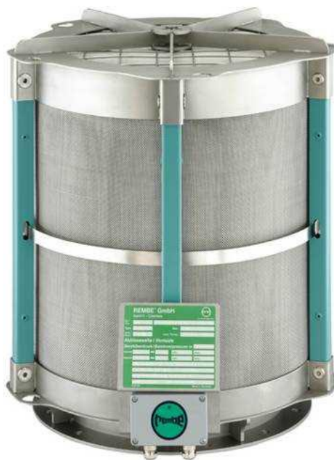
Figure 3. The Q-Rohr-3 flameless venting system from Rembe has an ATEX system certificate and can be installed indoors to safely vent an explosion.
