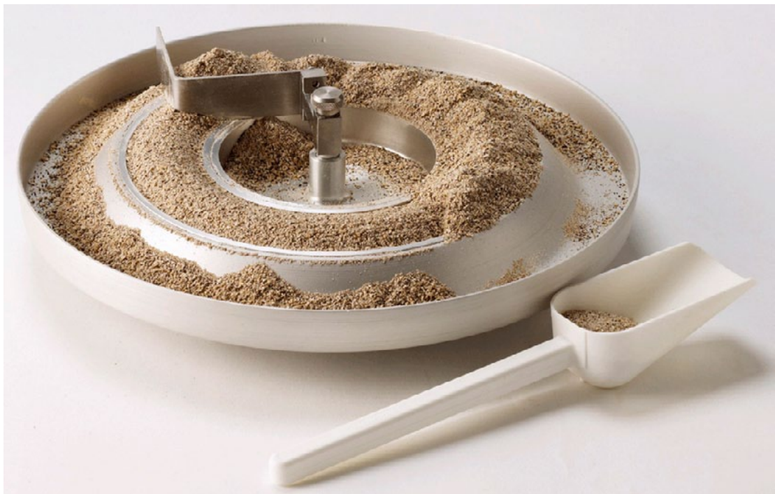
Figure 2: Powder is placed in an annular chamber or cell called a "trough" which is positioned on the shear cell instrument.
