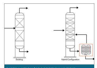
**DISTILLATION/ADSORPTION HYBRID** Figure 4. An adsorber can enable reintroducing a light component at an optimum location in a column, lowering energy consumption.
