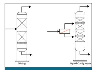
**MEMBRANE/DISTILLATION HYBRID** Figure 3. Using a membrane as a prefractionator frequently can provide substantial energy savings.
