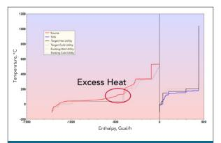
SURPLUS LOW-GRADE HEAT Figure 1. Complex 1 had the potential to supply very low pressure steam and hot water. Source: KBC.
