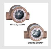
SFI-100 and SFI-300 sight flow indicators feature a removable window for easy service and replacement of wearing parts. The window also gives clear view of the rotating impeller, allowing an operator to easily view the direction and estimate the speed of flow.
