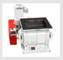
The MD has a cast housing and endplates with a square flange. The rotor and housing are precision machined to obtain a high degree of accuracy and close tolerances. Close tolerances hold the differential pressure across the valve to reduce air leakage. Reducing leakage saves supply gas, reduces spikes in velocity and stabilizes the system.
