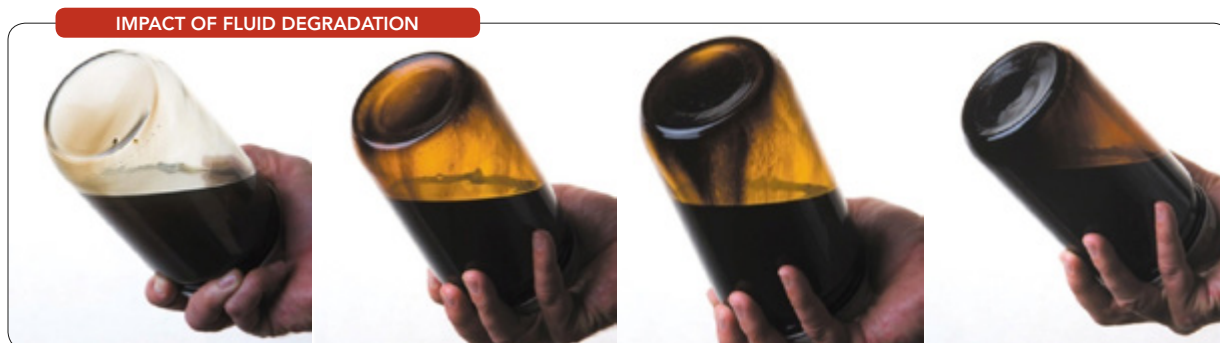
Figure 1. Fluid degradation either reduces the safety margin or increases the amount of maintenance required. Fluid degradation over time is inevitable; the goal is to minimize the rate at which it happens.
