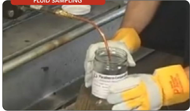
Figure 6. A properly performed fluid analysis is the most fundamental aspect of any routine maintenance plan for a thermal fluid system.
