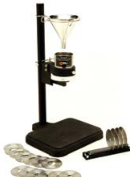
Figure 1. This apparatus provides qualitative data on solid's flow through orifices. Source: Hanson Research.
