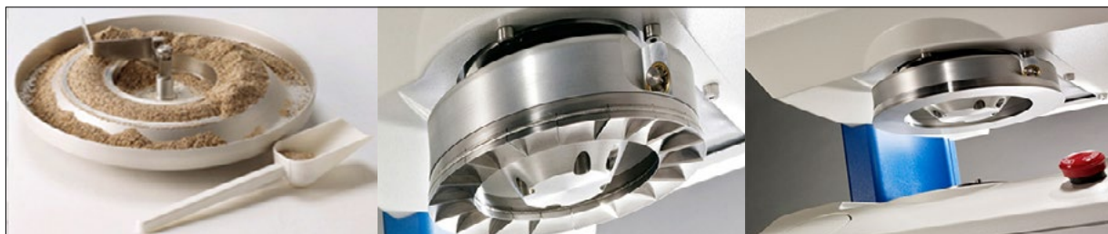
Figure 1: Annular shear cell components shown are a) trough with powder sample, b) vane lid and c) wall friction lid.
