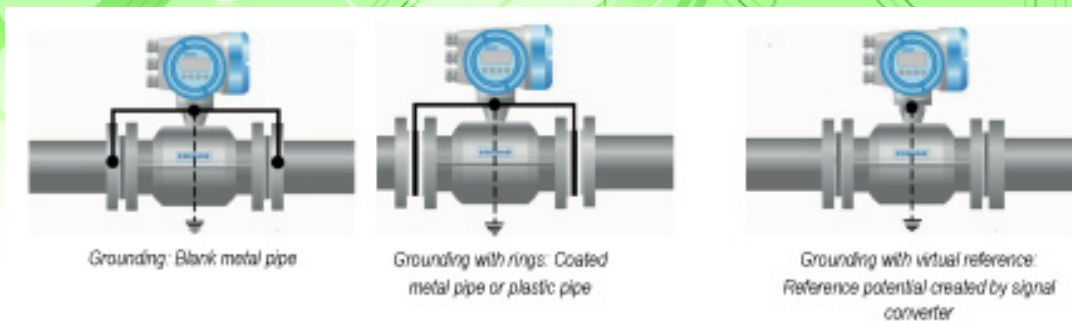
Figure 2. This diagram compares standard grounding methods with virtual reference.
