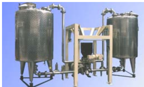
Powder induction from bulk bags in two process vessels with one Conti-TDS
