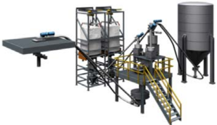
Figure 8. In this lime milling and blending system a tubular drag conveyor helps deliver the final product to a truck loading station..
