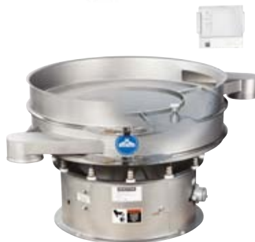
Figure 6A: The Ultrasonic screen cleaning system is installed in a round vibratory separator. The externally mounted electrical control box powers the transducer affixed to the screen tension ring. The screen is bonded to the exciter ring which vibrates the mesh.
