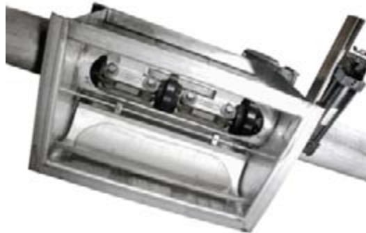
Figure 6. This full discharge gate valve features a convex valve design rather than flat, providing a tight seal to the conveyor with no internal gap.
