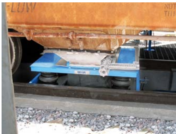
Figure 3. A CycloLift™ railcar connector elevates the boot from between the tracks and mates it firmly against the hopper slide gate — replacing conventional hydraulically activated mechanical linkages with pneumatically actuated lifters.
