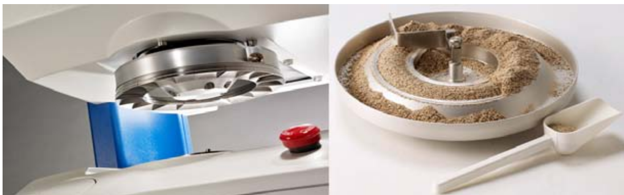
Figure 6: Shear cell components include a trough and vane lid.
