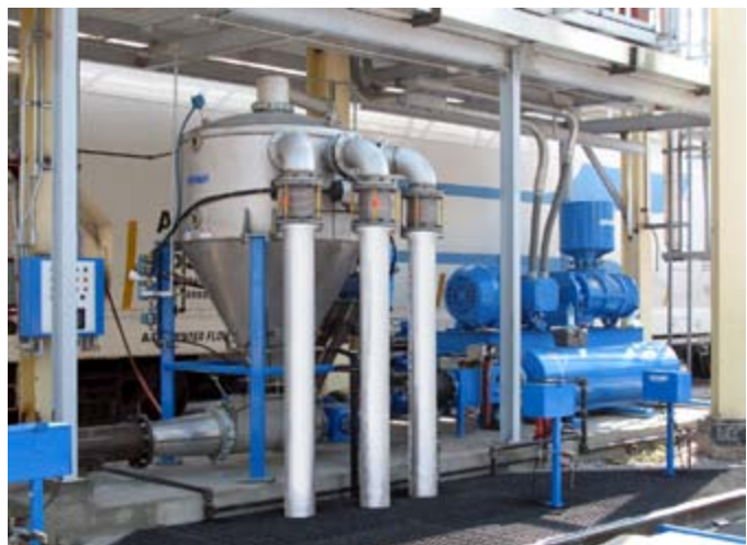
Figure 1. A vacuum-loaded Cyclonaire HC-75 semi-dense phase conveyor (high capacity – 75 ft 3 volume tank), with three material inlets, conveys materials at more than 25 tons per hour.
