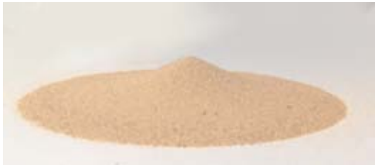
Figure 2: Dry sand forms a pile with "Angle of Repose" relative to horizontal.
