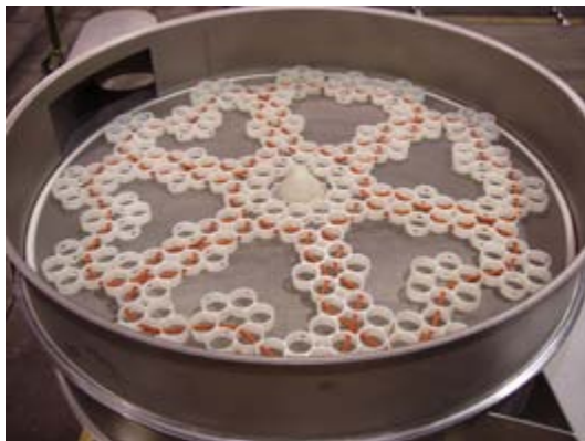
Figure 5: A top side wiper ring slides around on top of the screen to help clean the screen mesh openings.
