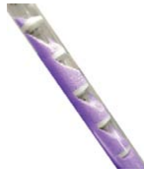
Figure 3. Tubular drag conveyor chain and flight assembly shown in a clear casing.
