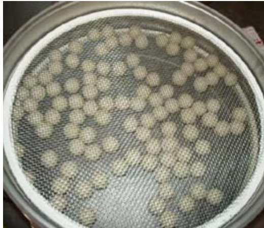
Figure 4: Self cleaning kit balls bounce between a support screen and the classifying screen. The vertical motion of the separator launches the balls and generates the screen cleaning action.
