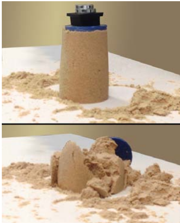
Figure 4: A 50g weight causes the sand castle to collapse.
