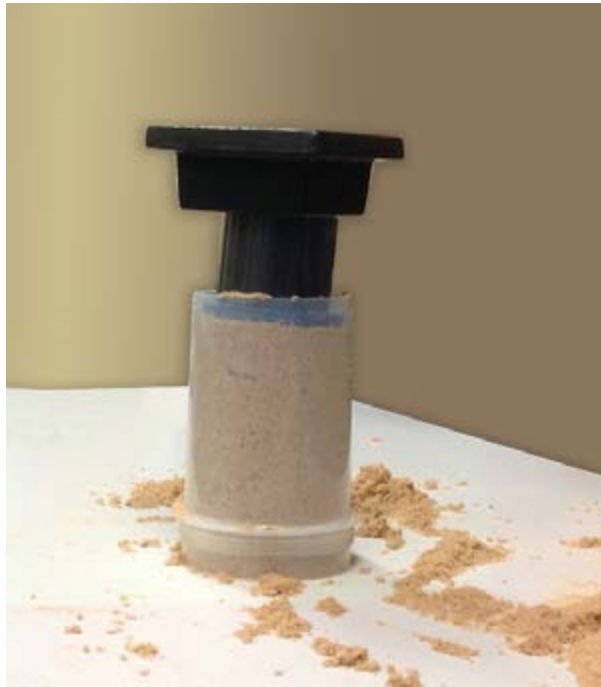
Figure 3: A 1kg Weight is placed on wetted sand causing consolidation.
