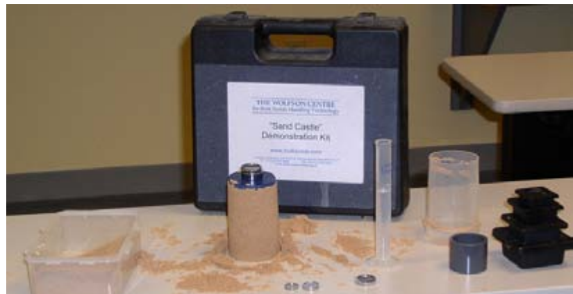
Figure 1: Sand Castle Kit for conducting uniaxial test.
