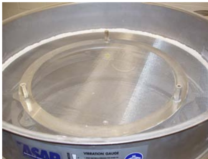
Figure 7: The screen energizer is attached below the screen surface.
