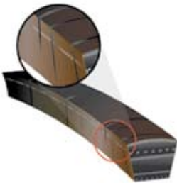
Figure 14 - Belt surface hard or stiff
