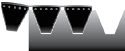
Figure 18 - Belt rib runs outside sheave
