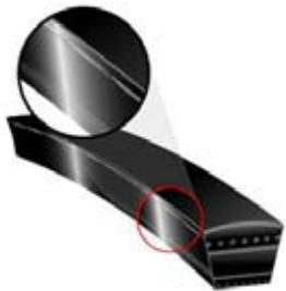
Figure 13 - Sidewall burning or hardening
