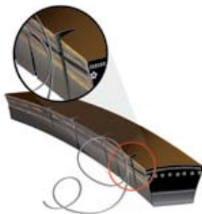
Figure 7 - Edge cord failure
