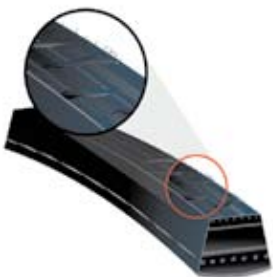
Figure 11 - Bottom surface wear
