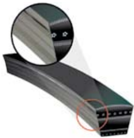
Figure 9 - Wear on belt sidewalls
