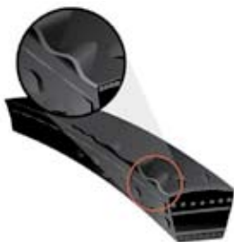
Figure 15 - Belt surface flaking, sticky or swollen
