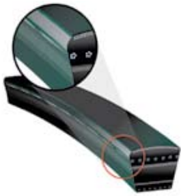
Figure 8 - Wear on top corners
