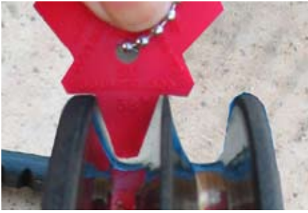
Figure 20 - An investigation into a customer's belt failure complaint identified this severely worn sheave.
