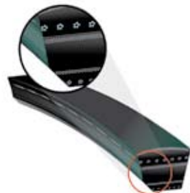
Figure 10 - Wear on belt bottom corners
