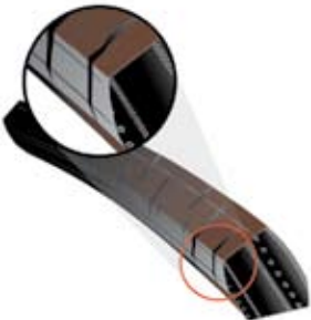
Figure 19 - Belt turns over or comes off sheave
