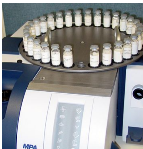
Figure 5 Vial autosampler for the MPA™ FT-NIR spectrometer.
