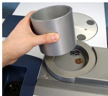
Figure 4 Placing a sample cup onto integrating sphere of the MPA™ FT-NIR analyzer.
