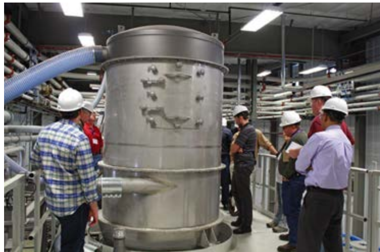
Figure 2. Vacuum systems use a system pressure lower than atmospheric pressure. They use a separator and a positive-displacement blower set between the vacuum charge side of the system and the pressure discharge side. Source: Kansas State Bulk Solids Innovation Center.
