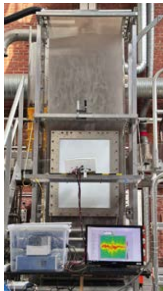
The Chalmers fluidized bed set up. The screen shows a real-time color map indicating the power intensity received, proportional to the solids concentration, and the velocity of the particles. Source: Chalmers University of Technology.
