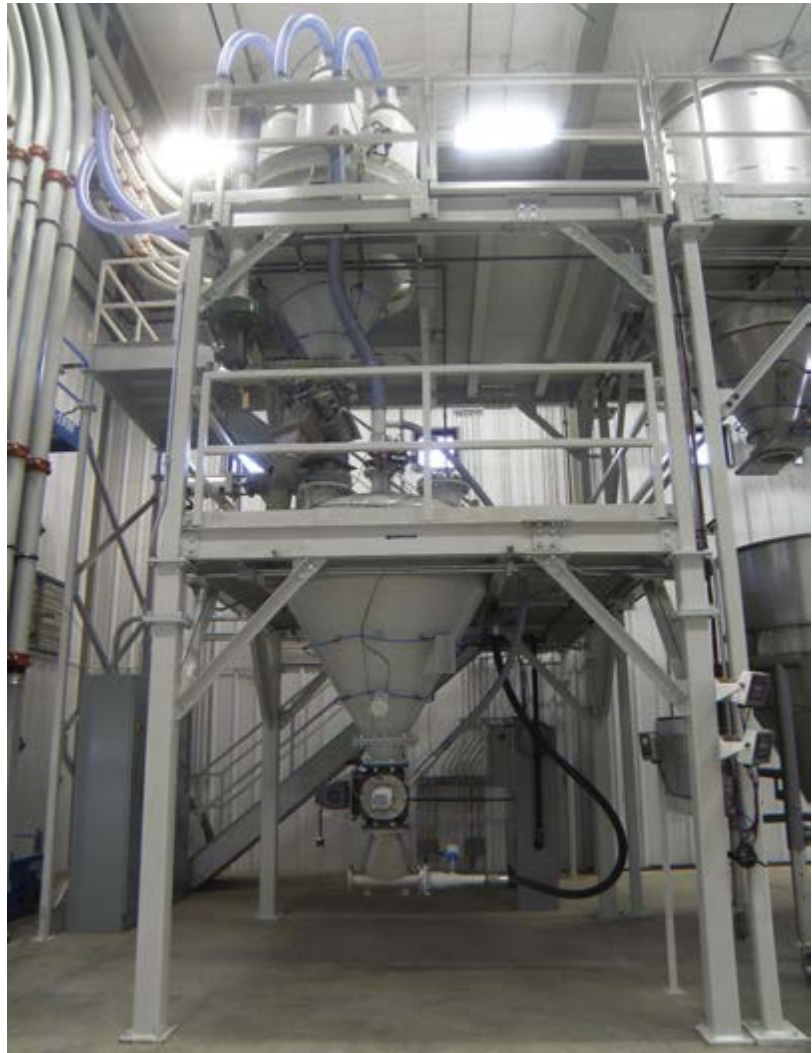
Figure 4. A dense-phase conveyor can handle materials such as different sands, feldspar, ashes, glass cullet, alumina, glass batch mix, carbon black, resins and beans. Source: Kansas State Bulk Solids Innovation Center.
