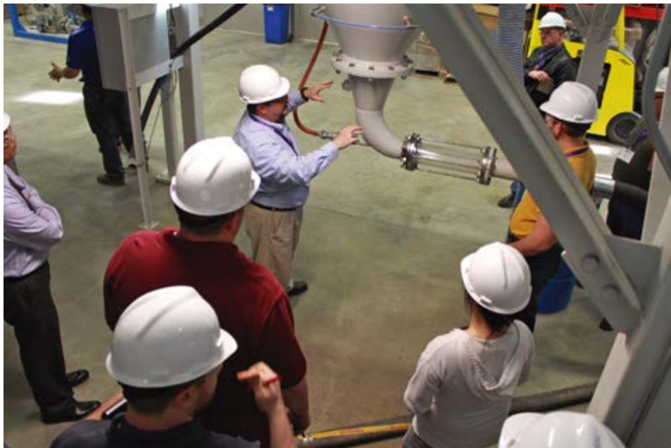
Figure 1. In pressurized or pressure systems, the bulk material is charged into an air or gas stream operated at higher than atmospheric pressures. Source: Kansas State Bulk Solids Innovation Center.
