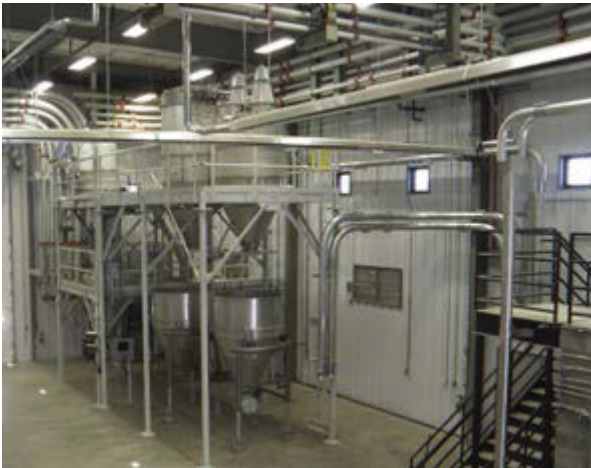
Figure 3. Dilute-phase conveyors move bulk materials suspended in an air stream from the positive pressure of a blower or fan set upstream of bulk material intake points or by a vacuum pump that removes air from the system downstream of bulk material discharge points.
