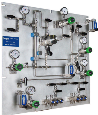
Figure 2. Adding modern gas pressure control panels to existing gas distribution systems allows maintenance technicians to more easily access components that need to be repaired or replaced.
