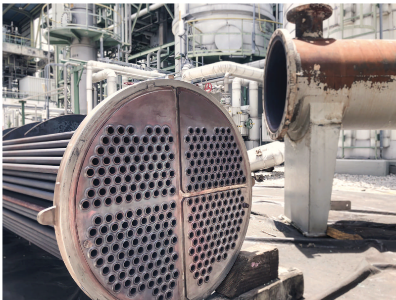
Figure 1. Shell-and-tube heat exchangers transfer heat by distributing the heating or cooling medium through the shell and heating or cooling the liquid through the tube, or in rare cases vice-versa.
