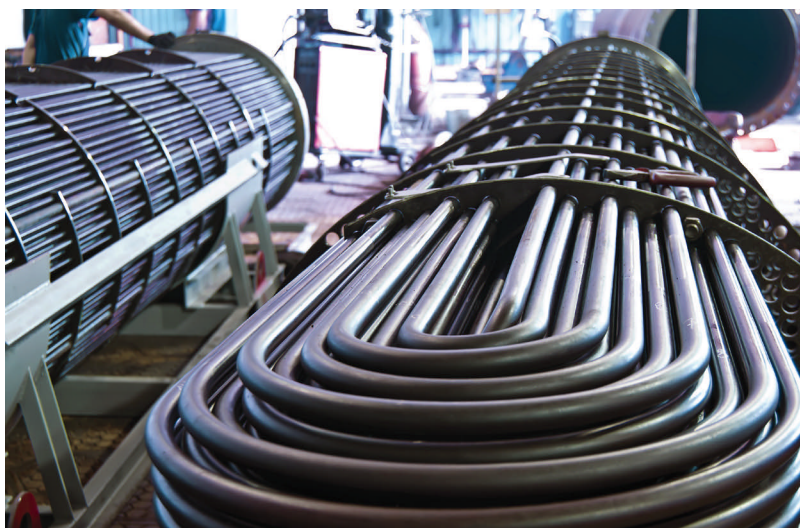
Figure 2. U-tube heat-exchanger designs allow for large temperature differences between the tube-side and shell-side fluids with the U-tubes expanding or contracting independently of the shell assembly.
