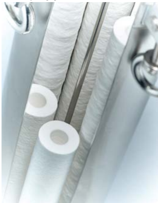
Figure 2. Loftrex Nylon filter cartridges in the housing. Levaco uses a total of 75 filter cartridges, spread across a 50-cartridge housing and a 25-cartridge housing. Source: Eaton Technologies
