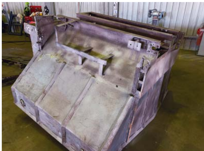
Figure 1. An example of a small hopper for bulk material handling under revamp and renovation at a workshop.
