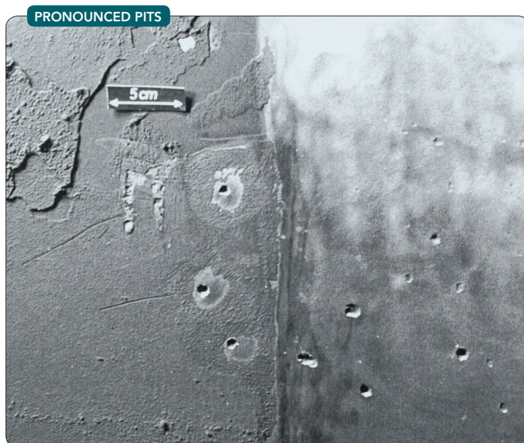
Figure 2. The inside surface of the column's duplex-stainless-steel bottom exhibited pits after five years in service.
