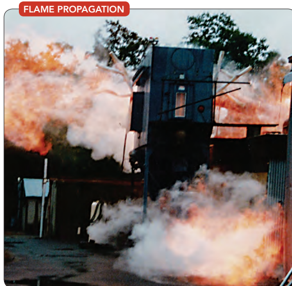
Figure 1. Highly energetic explosions can occur in connected equipment.
