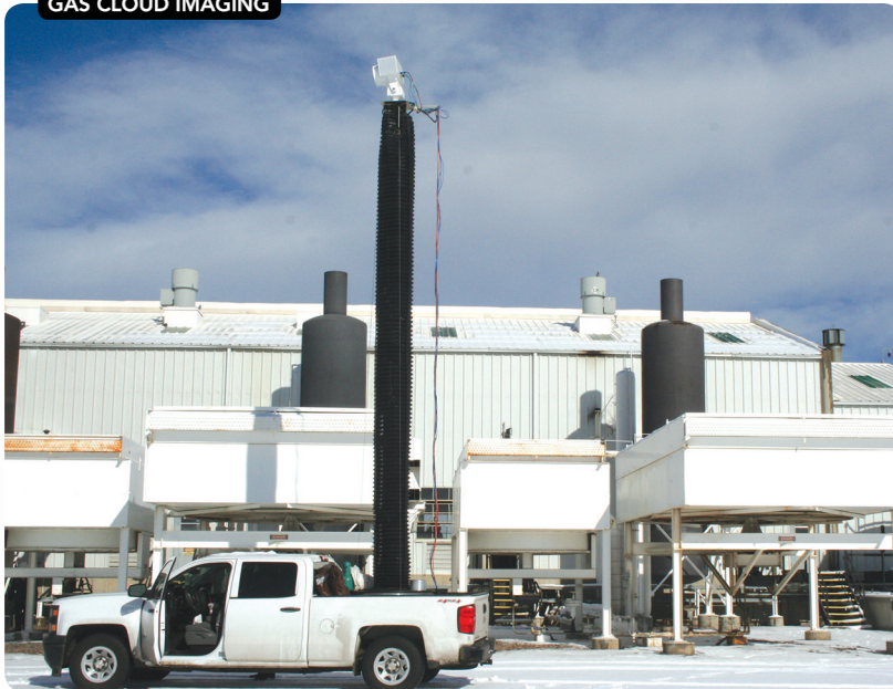
Figure 4. Camera can identify specific hydrocarbons and also generate a leak rate. Source: Rebellion Photonics.
