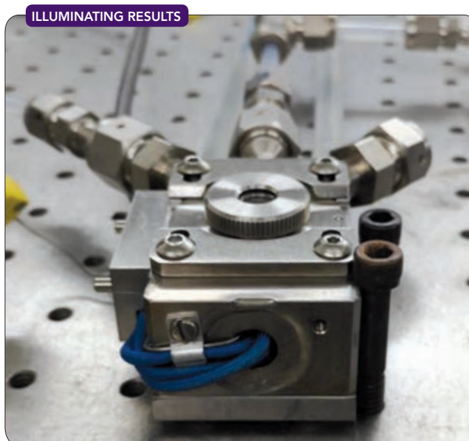
Figure 2. Laboratory reactor uses UV light to make methane with very high selectivity. Source: Duke University.
