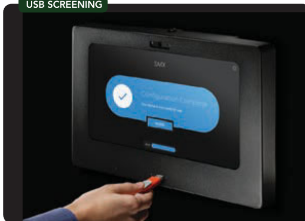
Figure 1. To be usable, USB flash drives must undergo checking by device at site. Source: Honeywell Process Solutions.
