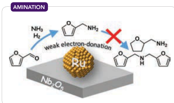
Figure 2. Highly selective catalyst consists of ruthenium nanoparticles on niobium pentoxide support. Source: Tokyo Institute of Technology.
