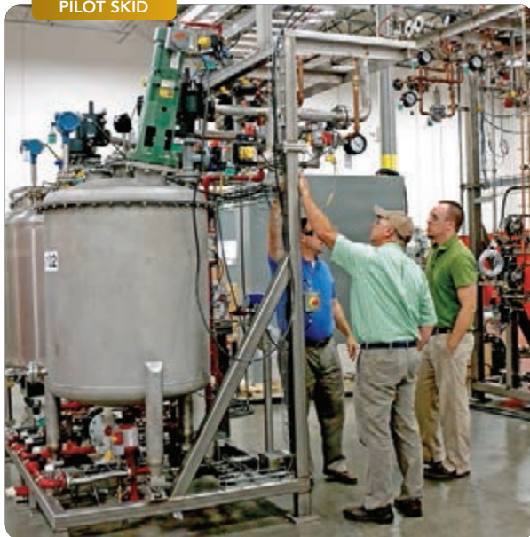
Figure 1. Off-site fabrication can improve the quality of pilot-plant elements and also compress the project schedule.
