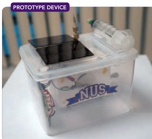
Figure 1. Solar-powered reaction of water and carbon dioxide to make methanol proceeds at ambient temperature and pressure. Source: National University of Singapore.
