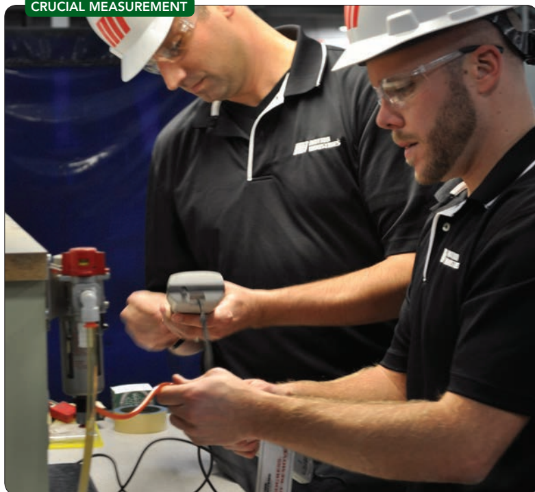
Figure 2. In-line hygrometer indicates the dewpoint of compressed air, which is part of assessing its operating condition.
