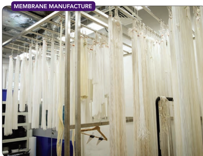
Figure 2. START Centre now is commercializing production of tri-bore membranes, shown here being dried. Source: National University Singapore.
