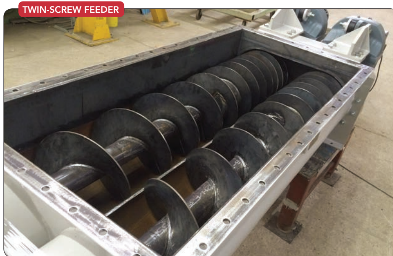
Figure 2. Unit features special extraction geometry and draws from the full width and length of the new hopper bottom.
