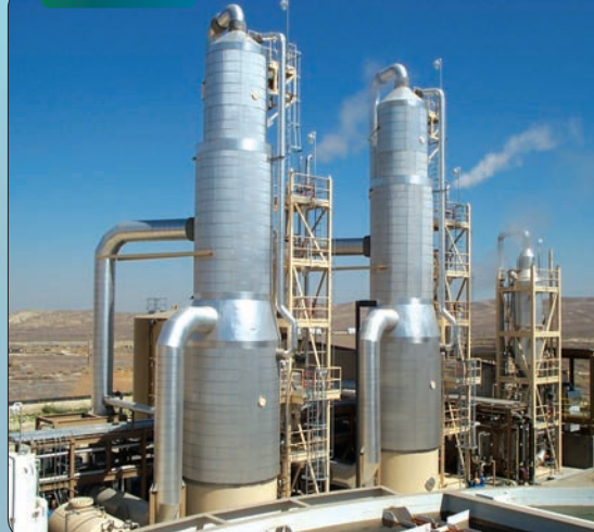
Figure 1. Making evaporator/crystallizer equipment smaller decreases opex and capex. Source: Suez Water Technologies & Solutions.
