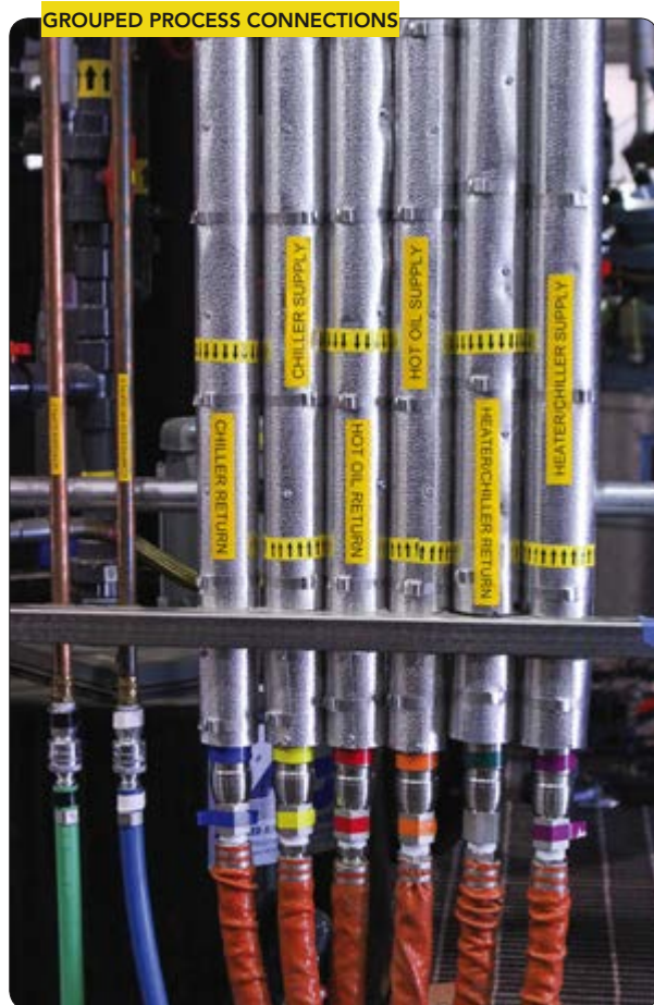
Figure 1. Such an arrangement simplifies initial hookups and, if required, later moving the skid to another location.
