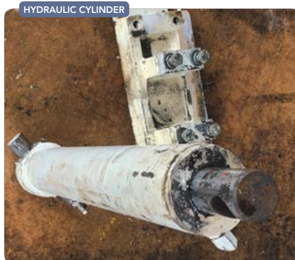
Figure 1. This heavy-duty double-acting unit awaits repair and refurbishment.
