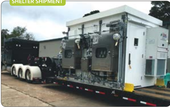
Figure 3. The cost and feasibility of transporting an analyzer shelter and installing it at the site can pose limitations.
