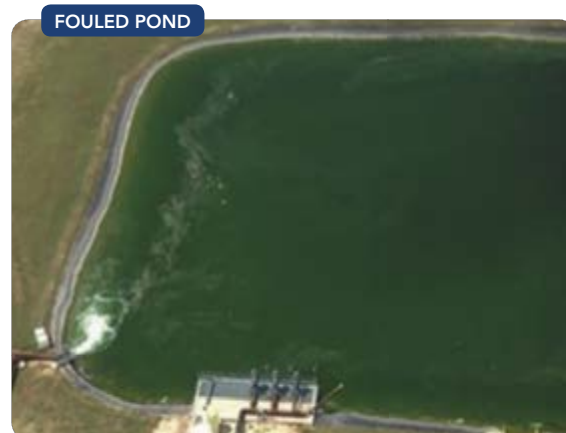
Figure 1. Phosphorus in return water fostered substantial algae and microbial growth.
