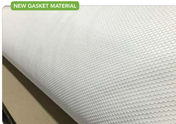
Figure 1. PTFE gasket features a raised hexagonal pattern that provides better compressibility.
