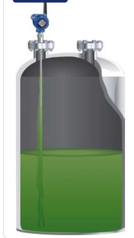
Figure 4. Buildup on a GWR probe eventually changes the profile of the echo in recognizable ways so operators become aware of the problem.
