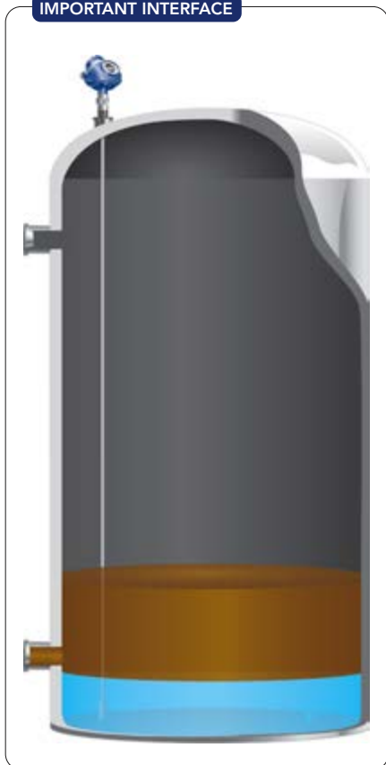
Figure 2. When emptying a tank filled with multiple liquids, knowing the interface level is necessary to avoid cross contamination.
