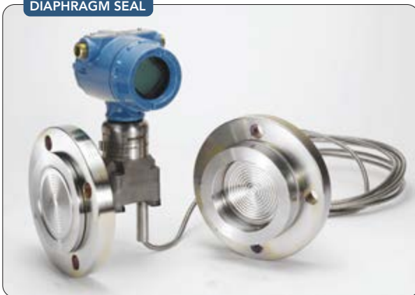
Figure 1. Such a seal uses a large diaphragm to transfer pressure to a fill fluid and prevents problems caused by process fluid directly contacting the instrument.
