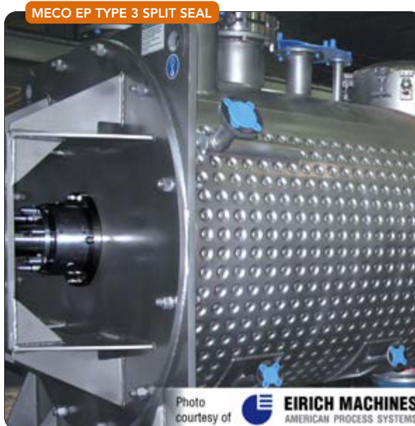
A Ø5" MECO EP Type 3 split seal on a cylindrical plow blender in service at temperatures approaching 500° F under full vacuum, drying calcium carbonate.
