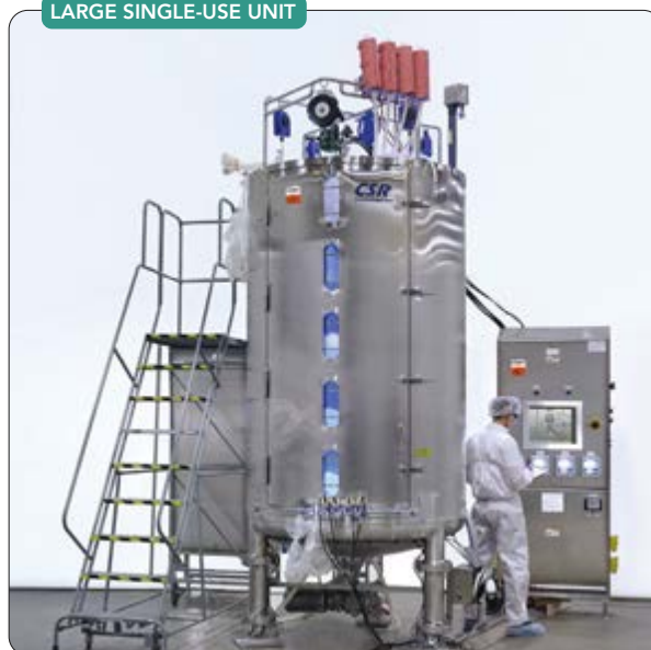
Figure 4. Chinese manufacturer has opted for 4,000-L disposable units at new commercial manufacturing facility. Source: ABEC.
