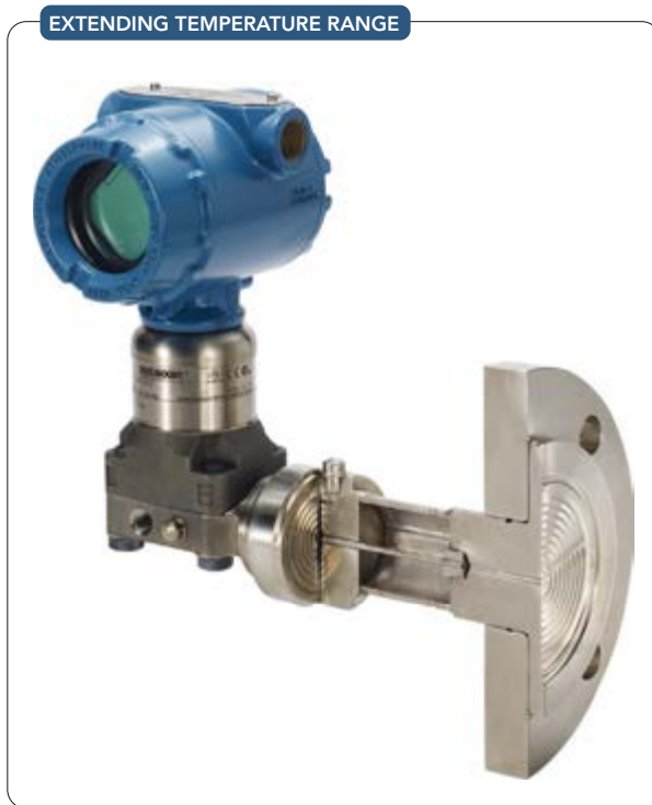
Figure 2. Process and ambient temperatures differing markedly may require use of a second fill fluid and, thus, an intermediate internal diaphragm.
