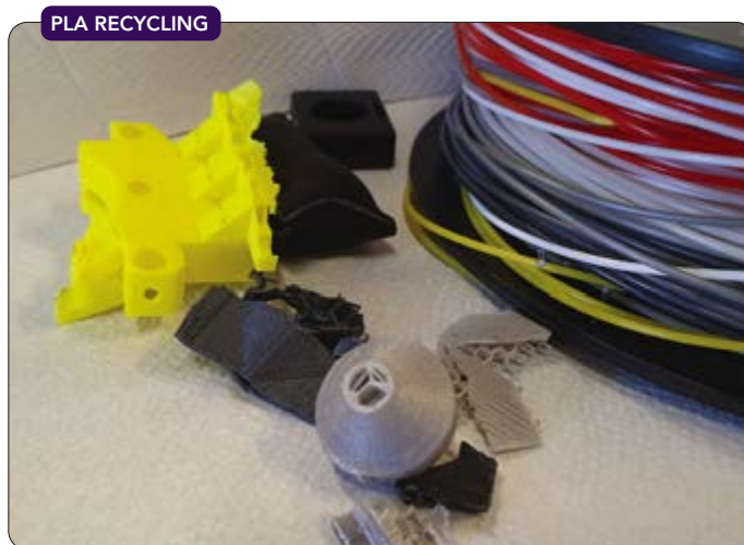
Figure 2. New catalyzed methanolysis process can turn 3D printer waste into methyl lactate. Source: University of Birmingham School of Chemical Engineering.
