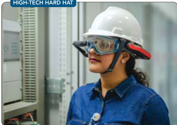
Figure 1. Lightweight unit features an intelligent built-in visual display and can capture and stream videos.
