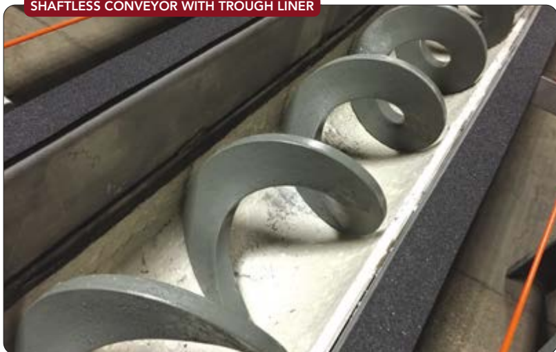
Figure 2. The ceramic lining enables smooth conveyance of wet or sticky materials. Source: KWS Manufacturing.
