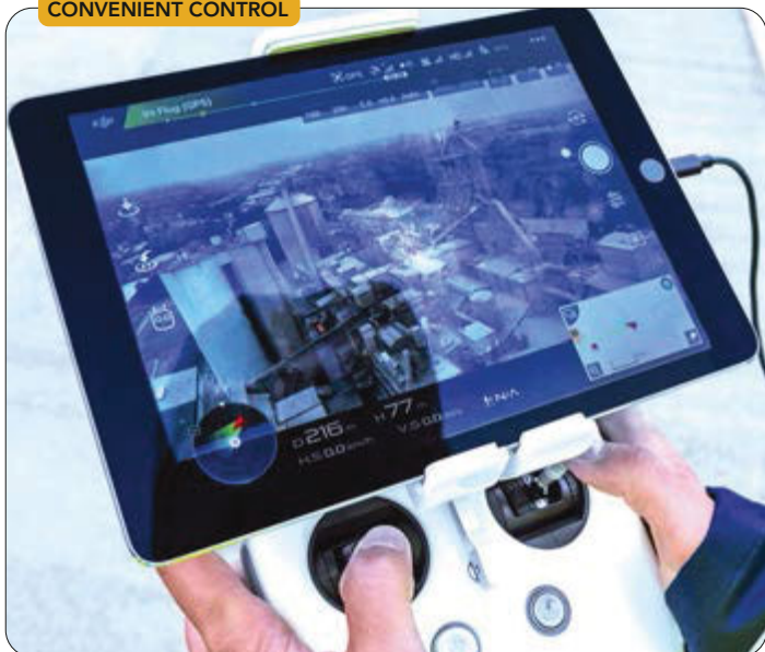
Figure 2. Hand-held unit can control drones sent out to detect issues and inspect equipment. Source: Thyssenkrupp.
